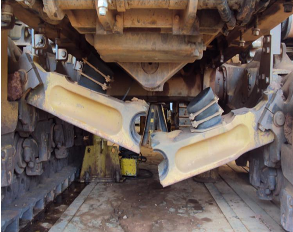
Figure 1. Equalizer bar after 500 hours in operation since inspection.
